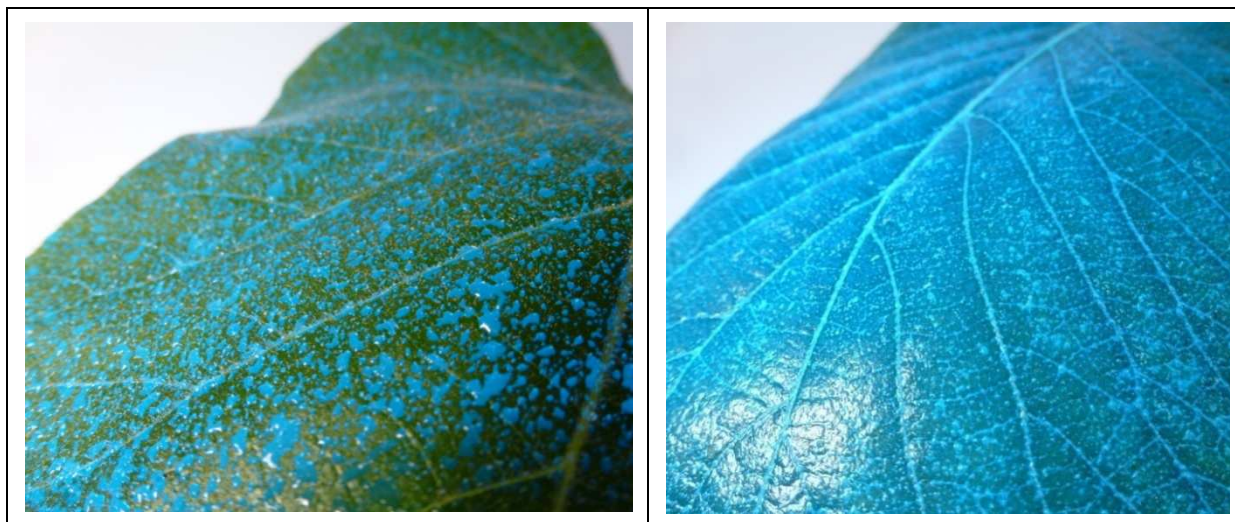
Photo 4: Coverage of a leaf top surface with (LHS) dilute spray containing Latron B, and (RHS) 3x concentrate spray containing Du-Wett superspreader (both sprays contain a UV dye to visualise deposits)
