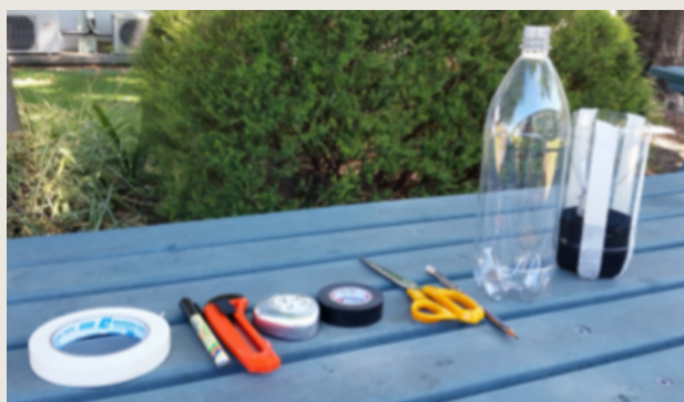
Before and after: all you need to make a light trap (left); completed home-made light trap (right).
