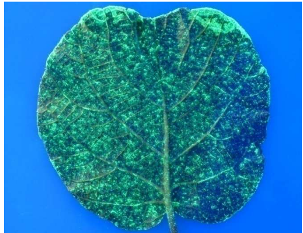
Fig. 26: Typical coverage of adaxial (top) and abaxial (bottom) leaf surfaces sprayed by ATR and AI nozzles.
