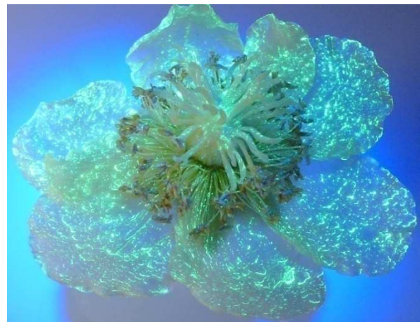
Fig. 25: Typical spray coverage of flower calyces and open flowers sprayed by ATR and AI nozzles.
