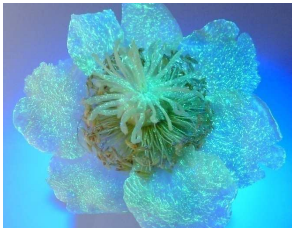
Fig. 25: Typical spray coverage of flower calyces and open flowers sprayed by ATR and AI nozzles.
