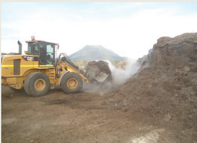
Left above: turning fresh green waste at Plateau Compost, Kawerau; and at right, turning a wind-row of compost containing reject kiwifruit.
